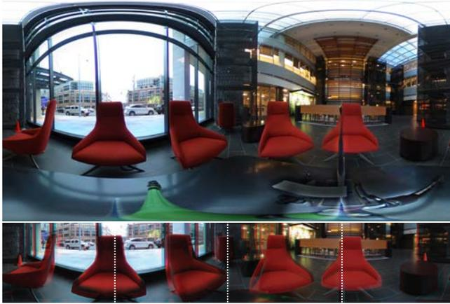
Fig. 11. Top: One image after geometric alignment. Bottom: An anaglyph illustrating the disparity offered by the uncorrected stereo pair. Note the correct disparity to the front (middle of equirect), vanishing stereo to the sides, and reversed stereo to the back (edges of equirect). Dashed vertical lines indicate  $\theta = 0, \pi/2, \pi, 3\pi/2$  for clarity.
